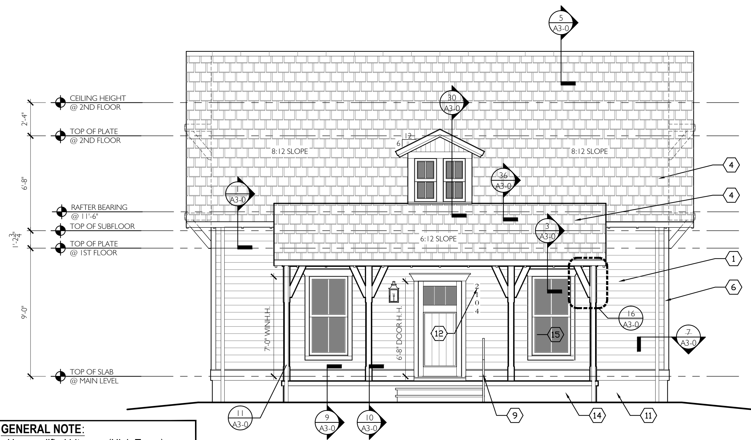
1 FRONT ELEVATION A2-1 1/4" = 1'-0"
